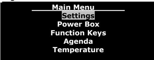
In the main menu, several menus can be opened. By using the arrow keys ↑ and ↓, the desired menu can be chosen and confirmed with "Enter".
