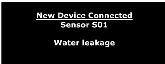
After connection, the control unit will display a Plug-In screen (Fig. 1), where a name can be assigned to the connected sensor.
