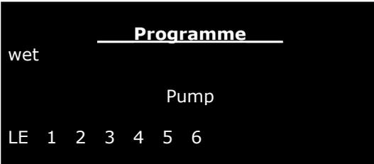
The example shown in Fig. 6 shows deactivation of socket "E" to which the ascent pump is connected every time the water leakage sensor takes on the "Wet" state.
